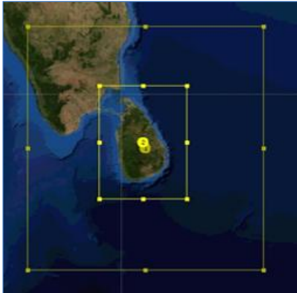
Fig. 2. Nested domains of the WRF model with resolutions of 12 km and 4 km (Source: Author's research)
