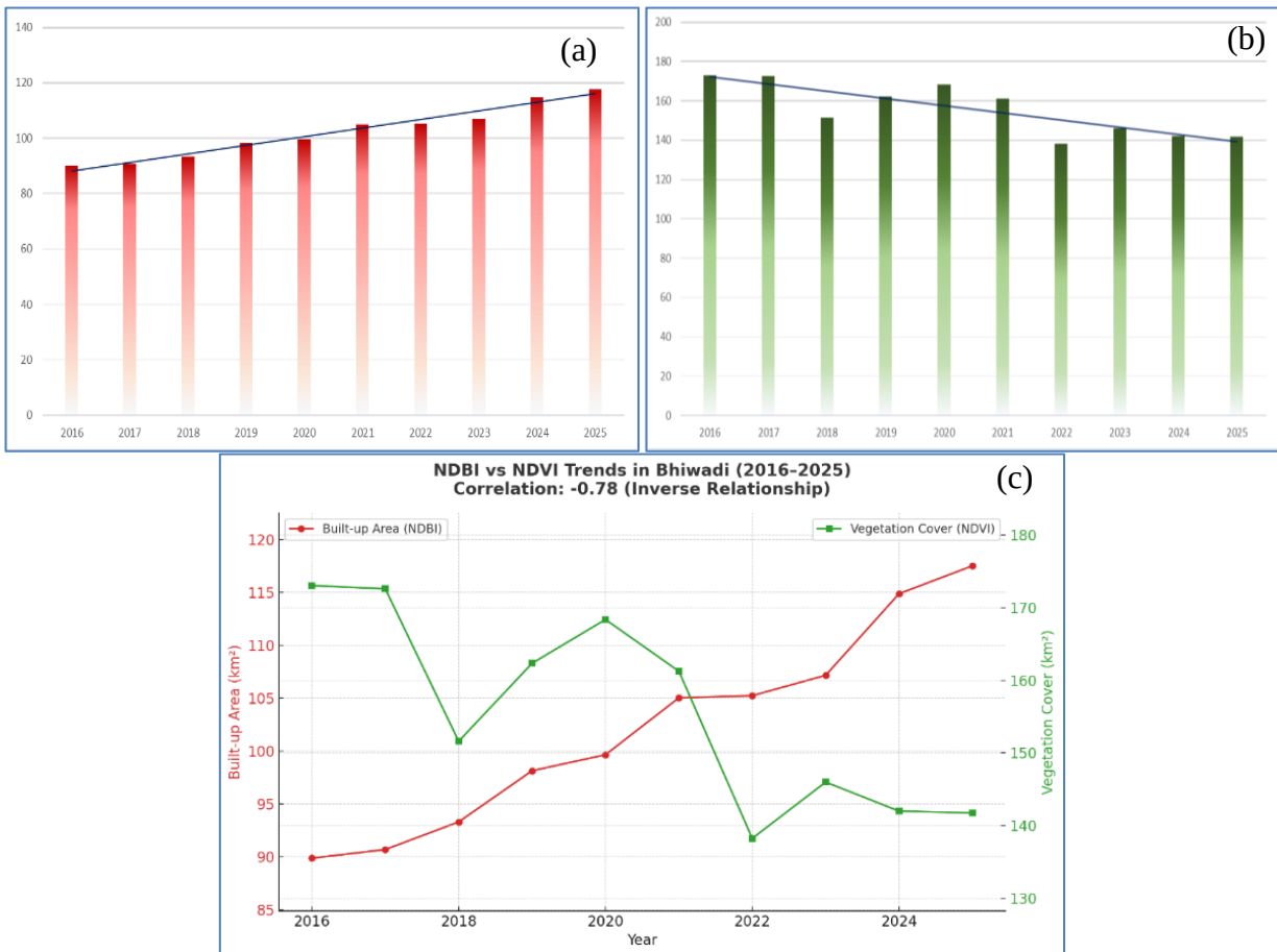
Figs. 5(a-c). (a) Annual variation in Normalized Difference Built-up Index (NDBI) for Bhiwadi from 2016 to 2025, (b) Annual variation in Normalized Difference Vegetation Index (NDVI) for Bhiwadi from 2016 to 2025 & (c) Correlation plot between NDBI and NDVI values (2016–2025) illustrating the inverse relationship between built-up expansion and vegetation cover decline
